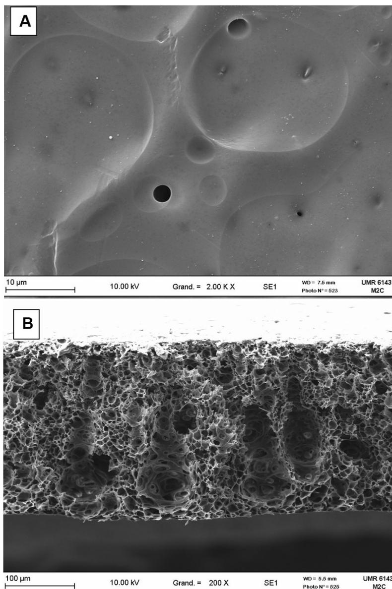
**Figure 2 :** SEM top-surface (A) and cross-section (B) of PSf/PAA 85/15 membrane
