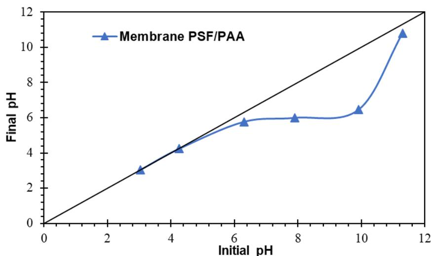
Figure 3 :  $pH_{PZC}$  (point zero charge) of PSf/PAA 85/15
