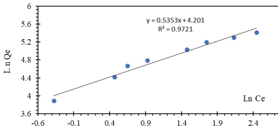
**Figure 10 :** Freundlich model for membrane PSf/PAA 85/15 at  $C_0 = 5 - 35$  mg/L,  $V = 100$  mL,  $m = 10$  mg, 120 rpm,  $\text{pH} = 10.5$  and  $T = 25 \pm 1$  °C.
