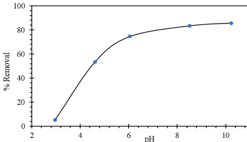
**Figure 4 :** Effect of pH on MB adsorption Onto PSf/PAA membranes.
