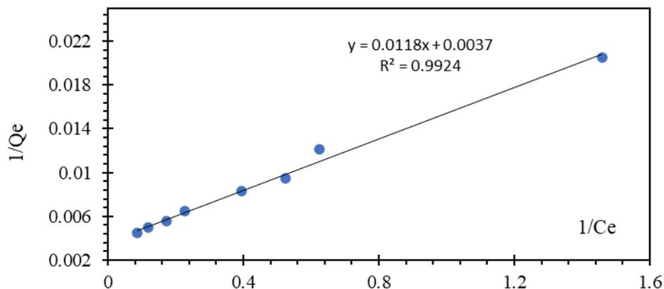
**Figure 9** : Langmuir model for membrane PSf/PAA85/15 at  $C_0 = 5 - 35$  mg/L,  $V = 100$  mL,  $m = 10$  mg, 120 rpm, pH = 10.5 and  $T = 25 \pm 1$  °C.
