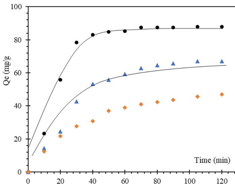
**Figure 5 :** Effect of membrane composition on MB adsorption
