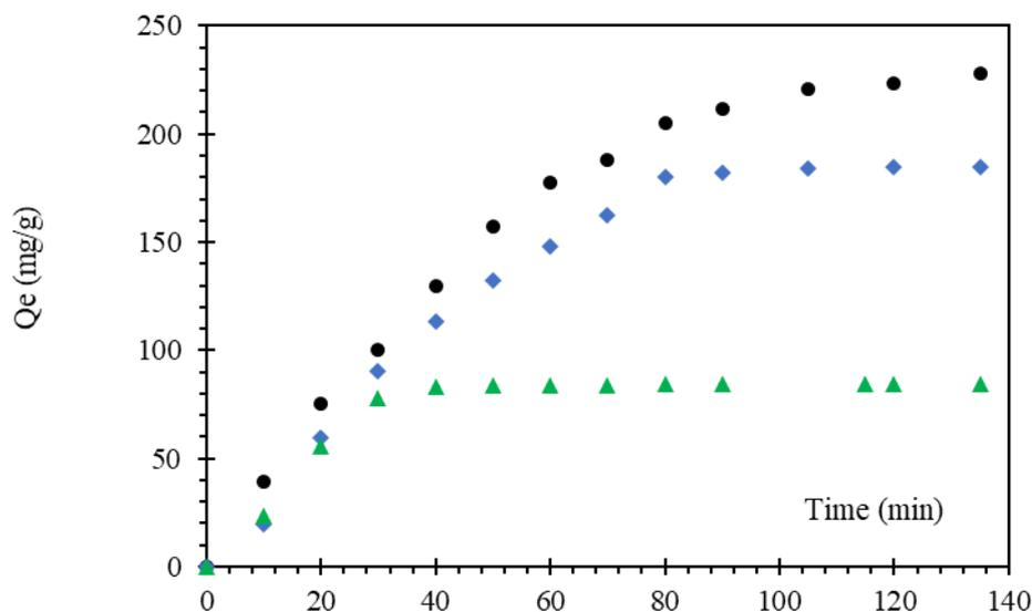
**Figure 6 :** Effect of dye concentration on MB adsorption onto PSf/PAA 85/15; (▲) 10, (◆) 25 and (●) 35 mg/L
