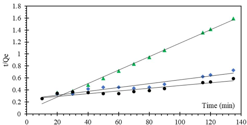
**Figure 8 :** PSO curves of the kinetics of MB adsorption onto PSf/PAA membrane at  $m = 10$  mg,  $V = 100$  mL, agitation speed = 120 rpm,  $T = 25 \pm 1$  °C and pH = 10.5.
