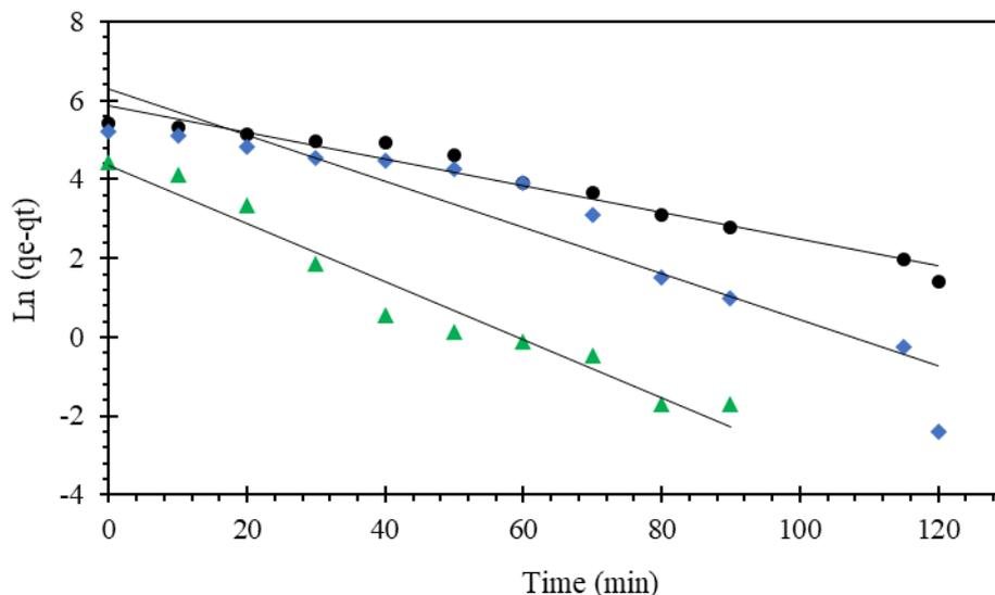
**Figure 7 :** PFO curves of the kinetics of MB adsorption onto PSf/PAA membrane at  $m = 10$  mg,  $V = 100$  mL, agitation speed = 120 rpm,  $T = 25 \pm 1$  °C and pH = 10.5.
