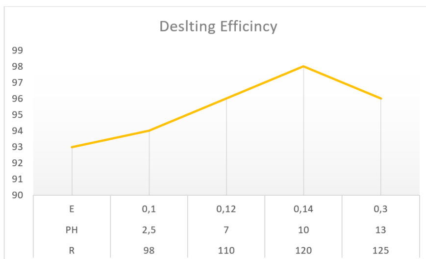
Figure 3. Optimum of desalting efficiency in function of key parameters
